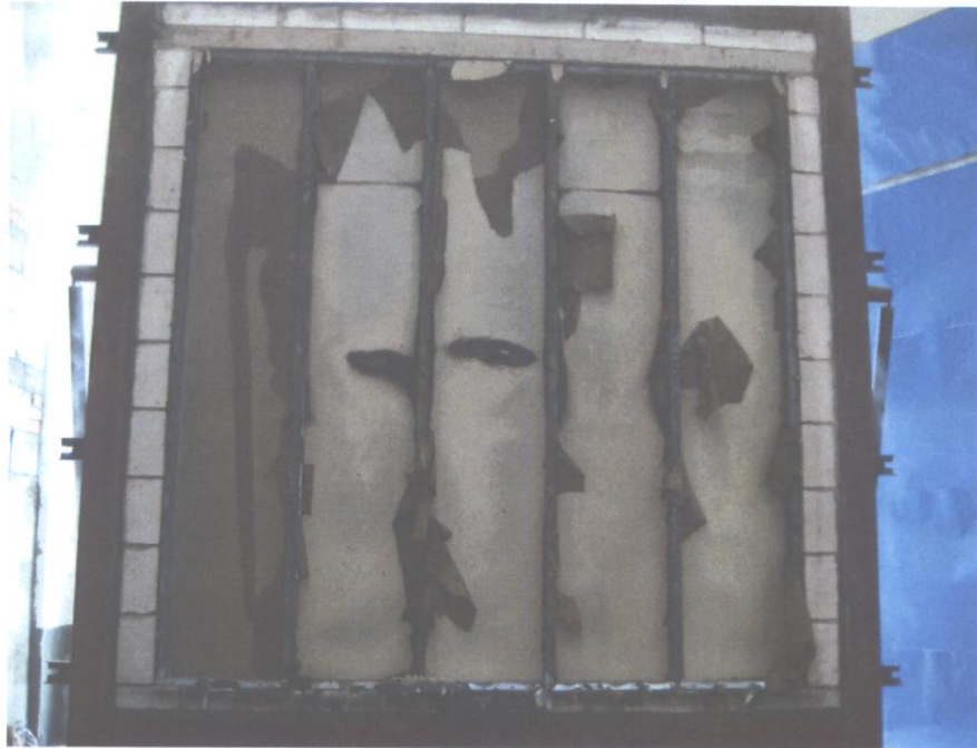
Fig. 9 – Exposed Side during Hose Stream Test
