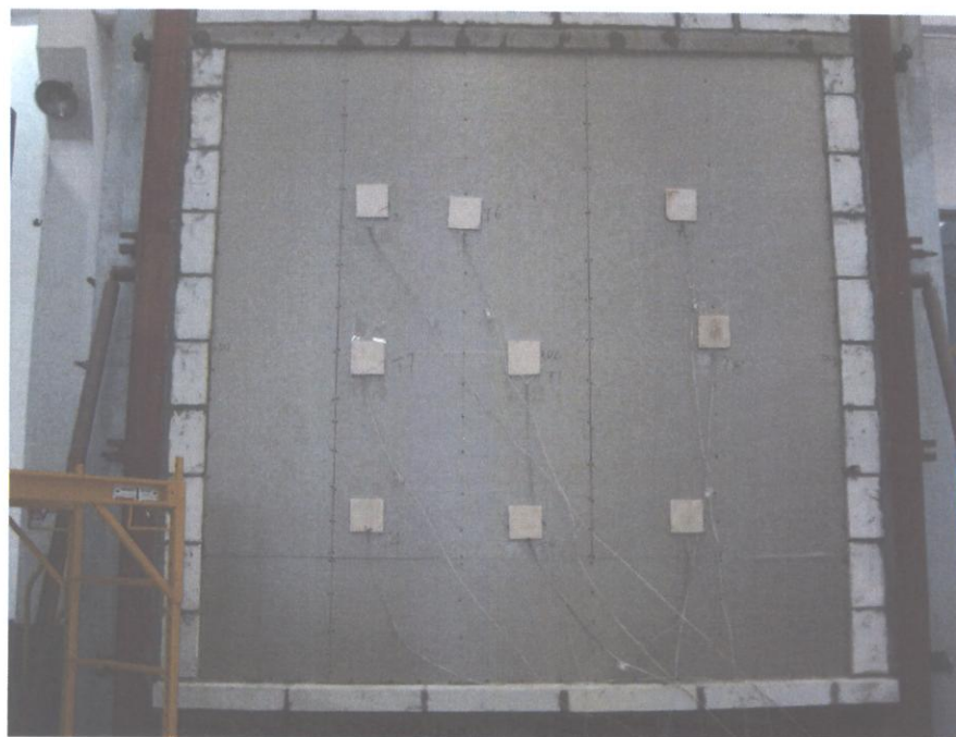
Fig. 5 – Unexposed Side after 90Minutes
