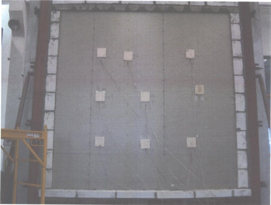
Fig. 4 – Unexposed Side after 60 Minutes
